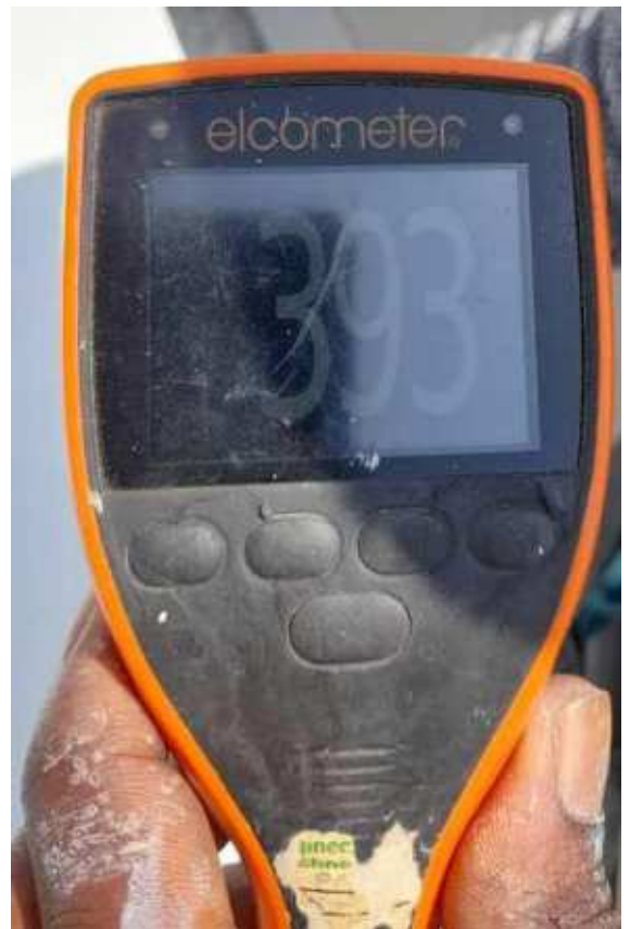
PART OF SOME OF OUR TEST EQUIPMENTS FOR ASCERTAINING SUBSTRATE SURFACE THICKNESS (DFT).
