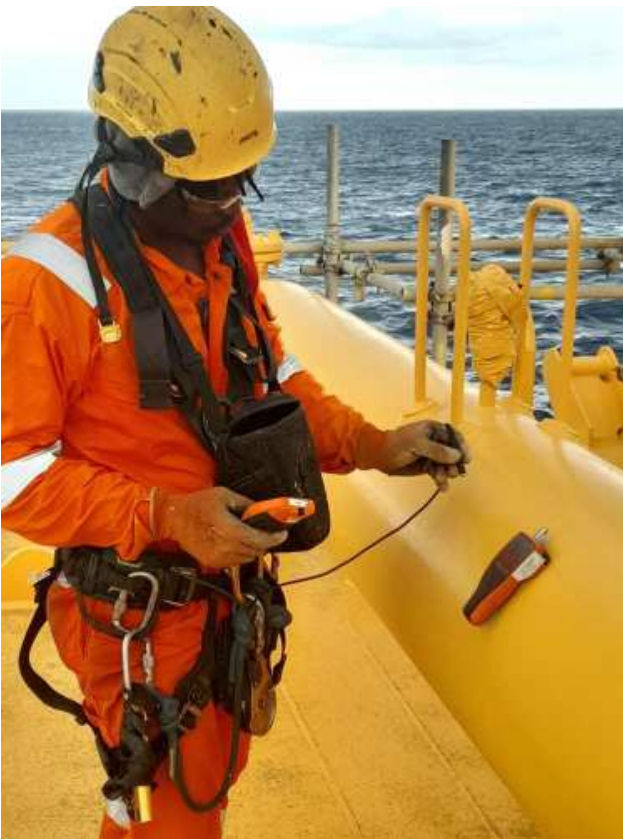
PART OF SOME OF OUR TEST EQUIPMENTS FOR ASCERTAINING SUBSTRATE SURFACE THICKNESS (DFT).
